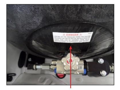
P/N: VWL ▲ DANGER ▲ VENTING OF THE PRESSURE FROM THIS SYSTEM REQUIRES THE USE OF SPECIAL INSTRUCTIONS OR TOOLS THAT CAN BE OBTAINED FROM VALVE MANUFACTURER OR ALTECH-ECO, (828) 654-8300.
